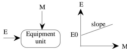
*Figure 2:5. A process equipment unit with its electricity demand function.*
