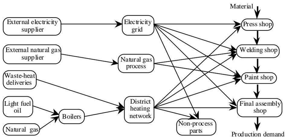
Figure 2:6. A schematic node network of the energy systems in Gent and Torslanda.
