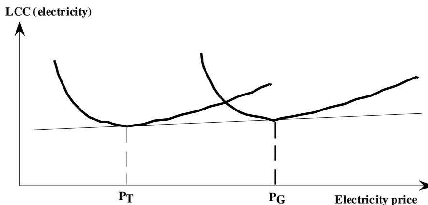
Figure 2:8. LCC for electricity use as a function of the electricity price for Gent ( $P_G$ ) and Torslanda ( $P_T$ ).
