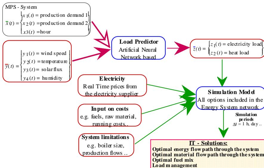
Figure 2:9. System architecture of an energy system integrated with other sub-systems within a company.
