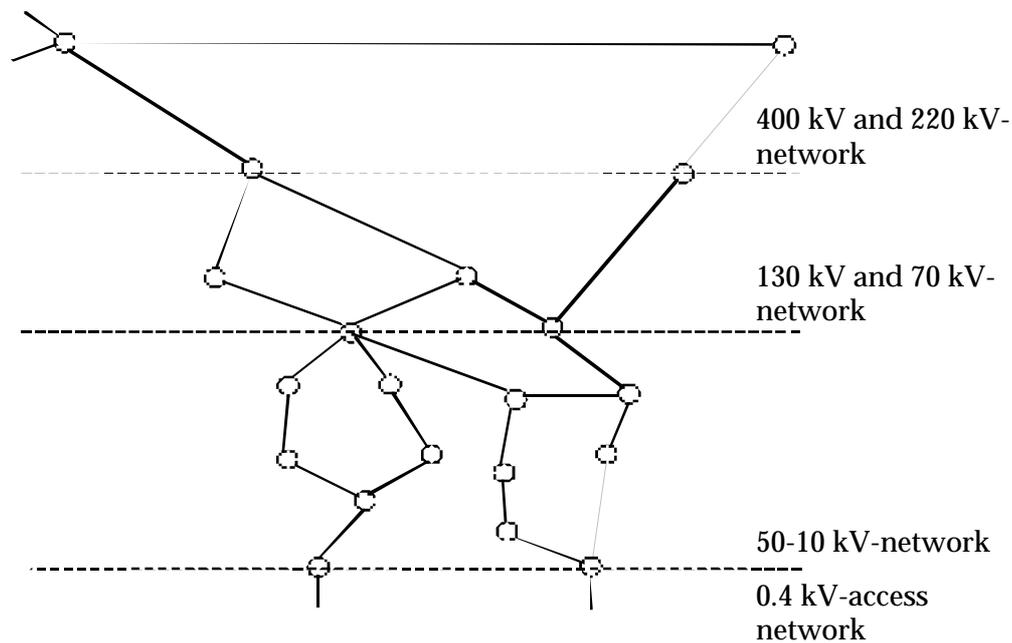
Figure 4:2. Configuration of the electric grid
