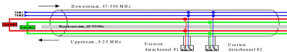
*Figure 4:1. Frequency usage in cable*
