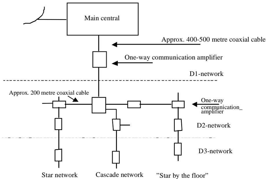
*Figure 4:4. Configuration of the cable-TV network*
