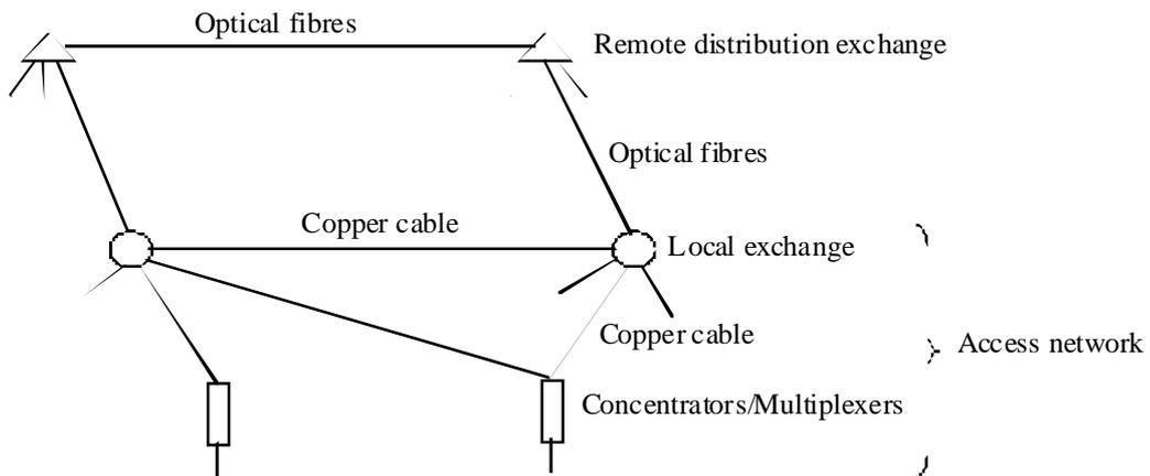
*Figure 4.8. Telecommunication network [8]*
