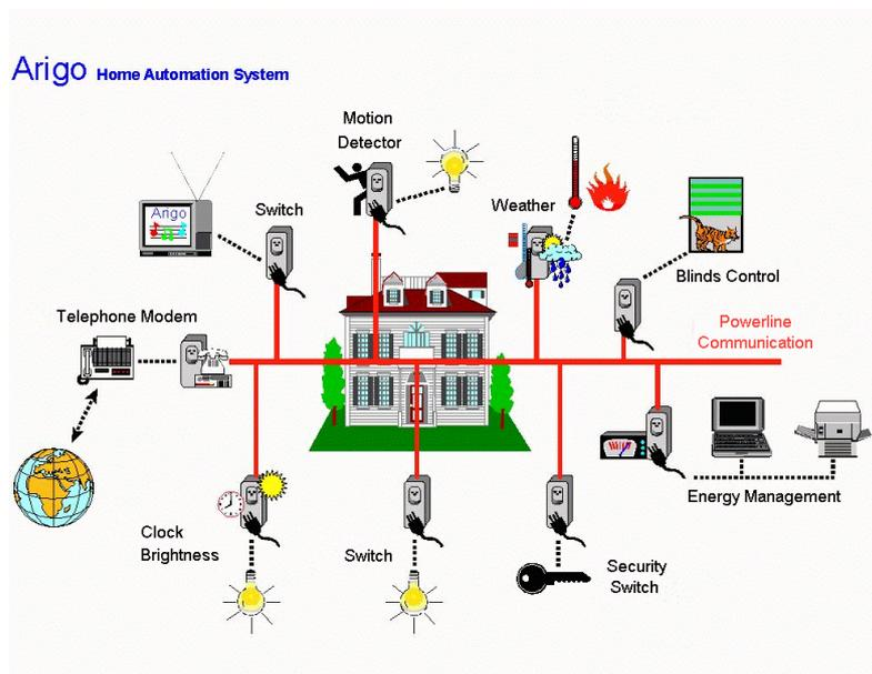
*Figure 5.2. Arigo system components connected to the power line.*
